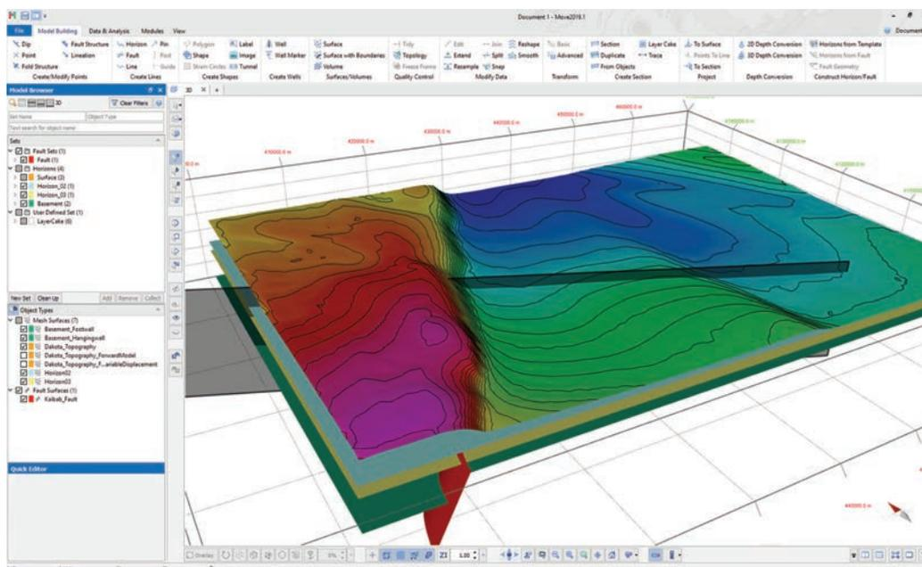
Discover the geological history of your modelled scenario to reveal unseen structures and changing geometries with our 3D Kinematic Modelling module. This module uses leading edge kinematic algorithms to validate and restore 3D geological models. Complex geological structures can be restored to identify alternative scenarios in areas of high structural uncertainty.
