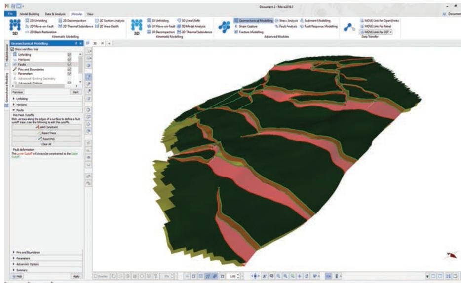
Our Geomechanical Modelling module uses elastic mechanical properties and physical laws of motion (Mass-Spring methodology, e.g. Wang et al. 2006) to mimic 3D rock deformation. Rapid modelling based on different geological assumptions can be done by running and saving multiple restoration scenarios with different mechanical properties, pin and fault displacement parameters.
