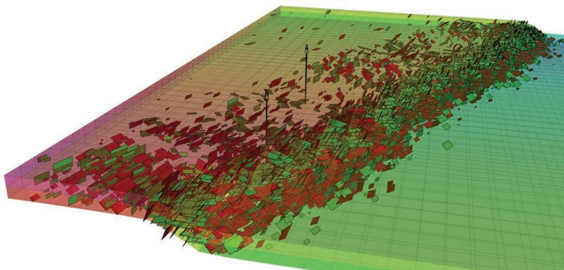
The Fracture Modelling module generates Discrete Fracture Network (DFN) models from an input geocellular volume. The workflow-driven approach guides users through the fracture modelling process, is easy to use, and facilitates rapid development of multiple fracture models. Combination with other MOVE modules (e.g. 3D Kinematic Modelling, Fault Response Modelling) provides a unique capability to build and test geologically valid fracture systems.
