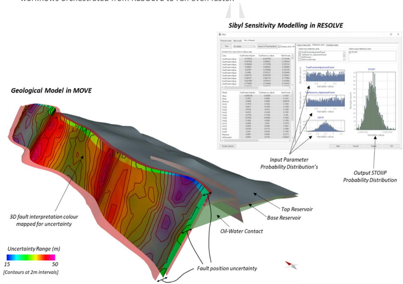
Use of the Sibyl sensitivity analysis tool to assess how uncertainty in the interpretation of structural features impacts volumetric calculations
