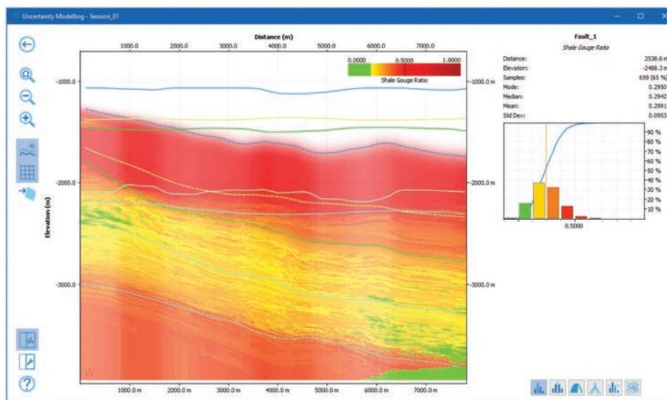
A tool for rapid evaluation of throw distribution, across-fault juxtaposition and fault sealing capacity in 3D. Combined with statistical analysis of fault displacement and scaling relationships, the tool provides powerful validation of geological interpretations.
