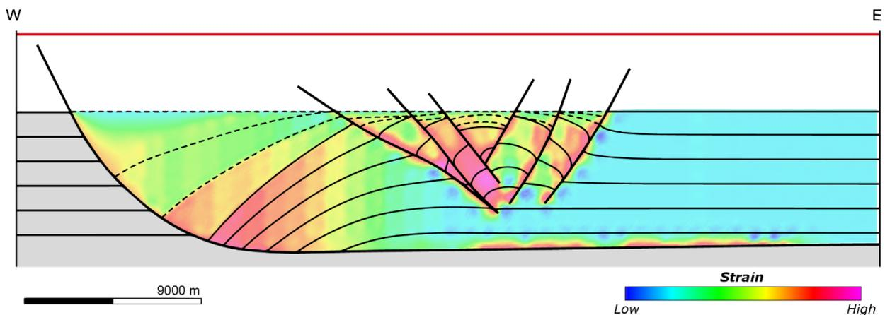
Figure 6. Forward model of crestal collapse in the hanging wall of a listric normal fault, colour mapped for strain intensity derived from the deformation of strain circles.
