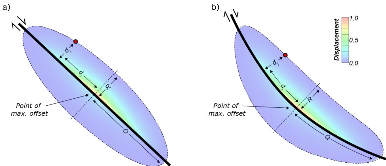
Figure 2. Illustration showing key parameters used to calculate displacement with Elliptical Fault Flow for: (a) a planar normal fault; (b) a concave upward curved, normal fault. Black dash lines represent the spatial extent of fault-related deformation. Area around faults colour mapped for the normalised displacement value, including 20% footwall movement.
