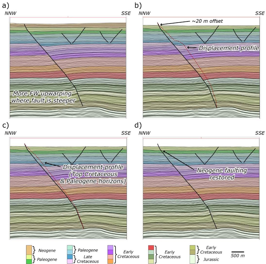
Figure 8. Restoration of a section through the Penobscot Fault, offshore Nova Scotia: (a) Present-day interpretation; (b) Removal of Neogene sediment with the amount of displacement along the fault visualised with red dashed line; (c) Removed Neogene with the amount of displacement along the fault defined by Top Cretaceous and Paleogene horizons visualised with red dashed line; (d) Restoration of Neogene fault slip. Seismic data from Nova Scotia Department of Energy.
