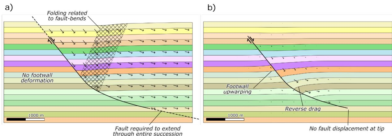
Figure 1. Forward models of normal fault using: (a) inclined Simple Shear with approximately uniform displacements in the hanging wall; (b) Elliptical Fault Flow, with displacements that decrease away from the centre of the fault.
