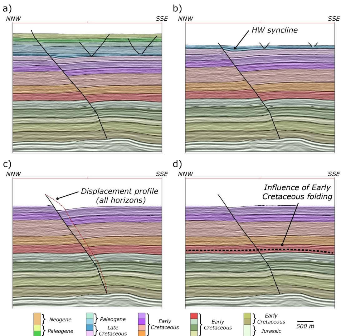
Figure 9. Continued restoration of a section through the Penobscot Fault, offshore Nova Scotia: (a) Restoration of Neogene fault slip; (b) Removal of Paleogene sediment; (c) Removal of Late Cretaceous sediment with the amount of displacement along the fault visualised with red dashed line; (d) Restoration of Late Cretaceous fault slip. Seismic data from Nova Scotia Department of Energy.
