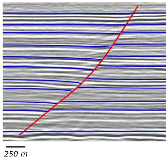
Figure 5. Horizons around an isolated normal fault in the Bryant Canyon area of the Gulf of Mexico that have been forward modelled with **Elliptical Fault Flow** to match seismic data. Seismic data is taken from the National Archive of Marine Seismic Surveys (Triezenberg et al. 2016).
