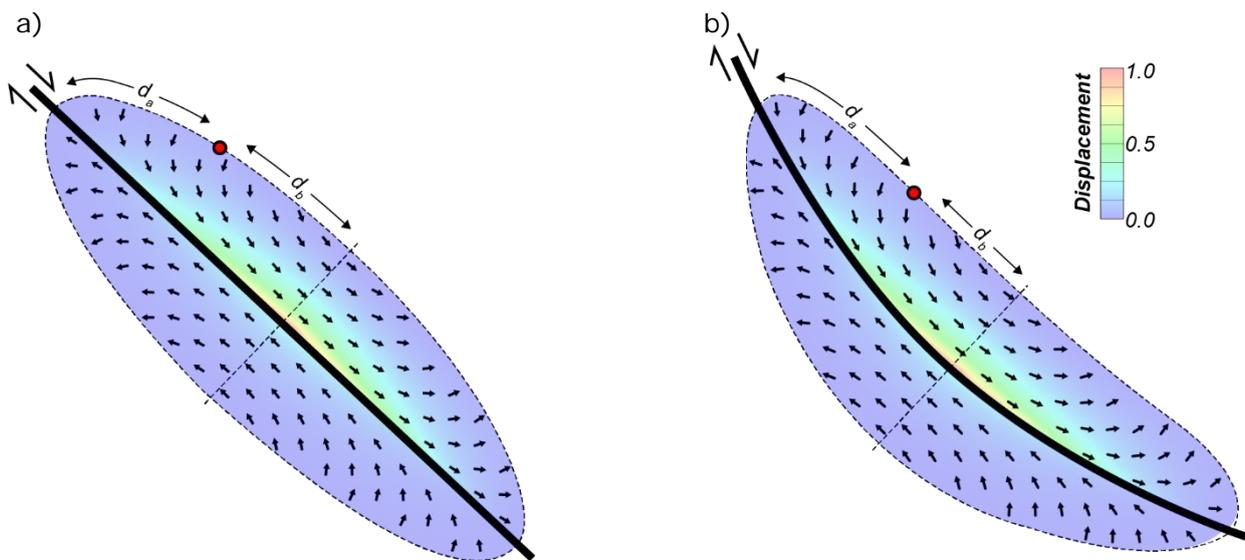
Figure 3. Illustration showing the normalised deflection factor and maximum possible deflection of movement trajectories (Maximum Deflection Angles of 90 degrees) around: (a) a planar normal fault; (b) a concave upward curved, normal fault.
