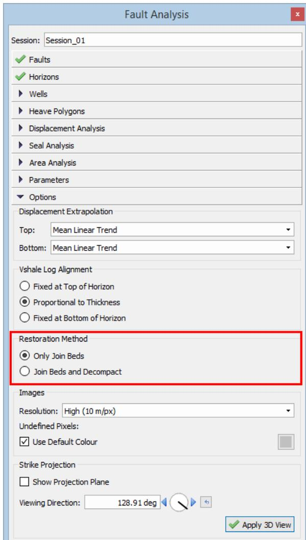
Figure 7. Restoration Methods on the Options sheet.
