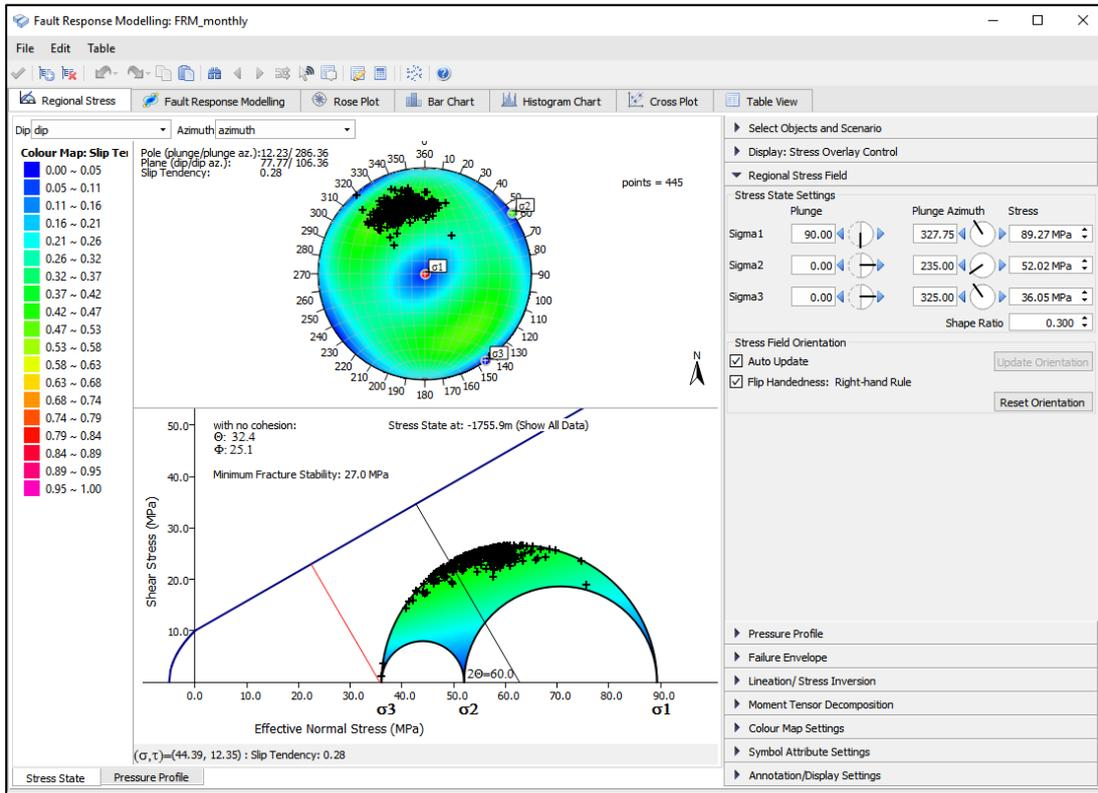
Figure 4. The Regional Stress sheet in the Fault Response Modelling interface
