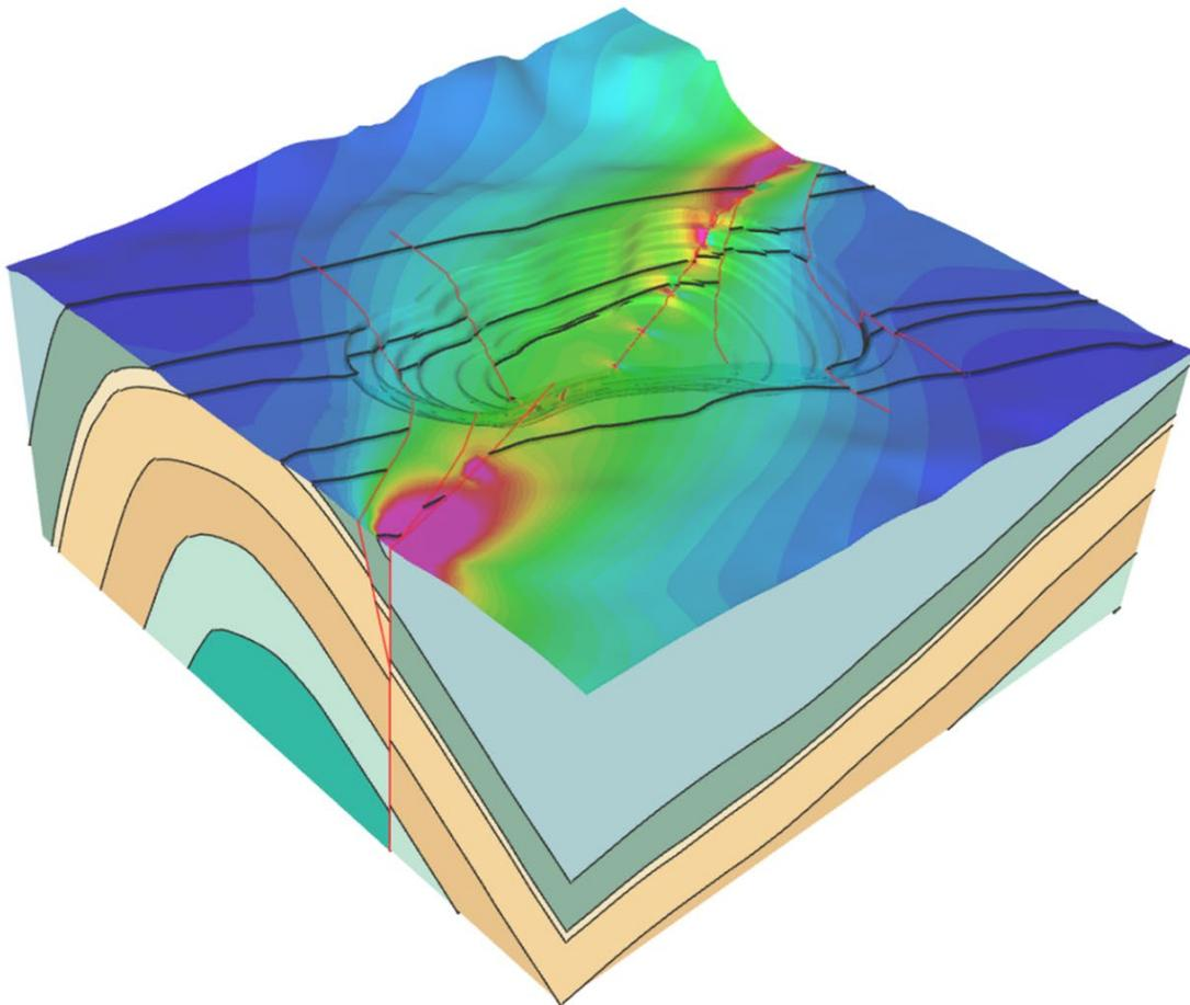
*Figure 1. A 3D model in Move – geological model built and DEM colour mapped for strain associated with faulting. As discussed in this feature, this type of analysis can be important in mineral exploration and mine planning.*
