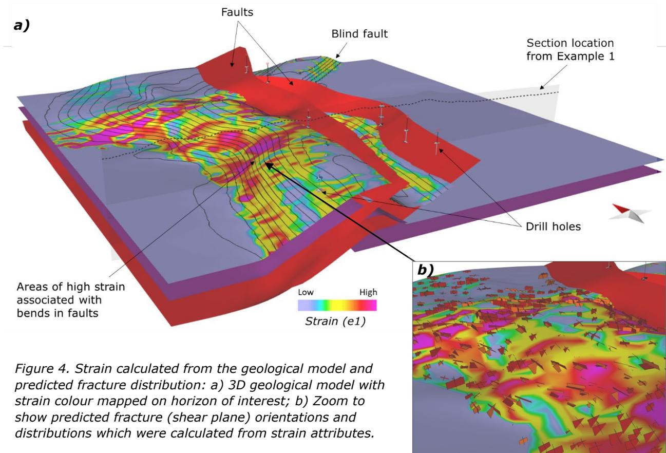
Figure 4. Strain calculated from the geological model and predicted fracture distribution: a) 3D geological model with strain colour mapped on horizon of interest; b) Zoom to show predicted fracture (shear plane) orientations and distributions which were calculated from strain attributes.
